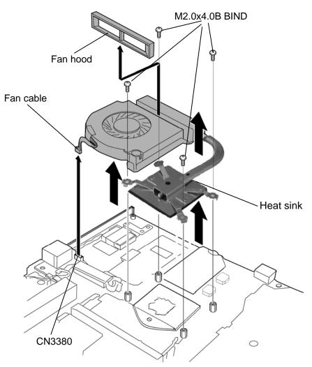
Figure 4-31 Removing the heat sink (with fan)
